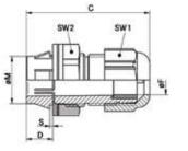
SKINTOP<sup>®</sup> CLICK is an innovative cable insertion system that provides fast, highly flexible assembly. Easy snap-in-place installation results in fixed, centered, strain relief with maximum protection in seconds. Mounting hole is based on metric thread. SKINTOP<sup>®</sup> CLICK-R includes reducer bushing.
