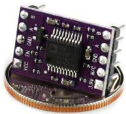
Basic EZO™ Inline Voltage Isolator
