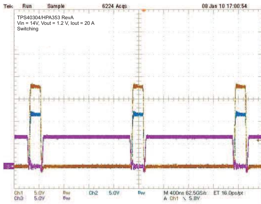
Figure 8. TPS40304EVM-353 Switching Waveforms
