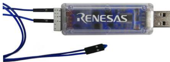
Figure 1. DAQ on a Stick with Semitec RTD Temperature Sensor
