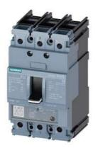
circuit breaker 3VA5 UL frame 125 breaking capacity class S 25kA @ 480 V 3-pole, line protection TM230, FTAM, In=60A overload protection Ir=60A fixed short-circuit protection li=5...10 x In cable connection on both sides
