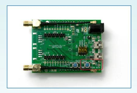
Users may use SW2 to turn off the modem or to turn the modem back on after a shutdown when the automatic turn on circuit is enabled.
