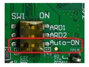
Users may also manually turn the modem on or off by disabling the auto turn on circuit by setting SW1-3 to the off position and then use SW2, labeled "ON BTN" on the circuit board, to manually pulse the modem's ON\_OFF line low.
