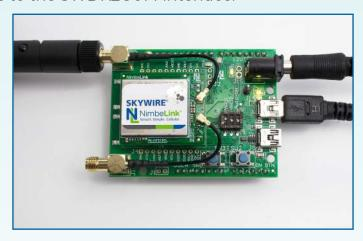
The J14 interface will connect to the modem's USB to serial UART interface IC to access the modem's serial UART interface. The D3 LED will illuminate when USB is connected.
