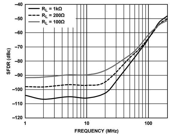
Figure 36. SFDR vs. Frequency for Various Loads
