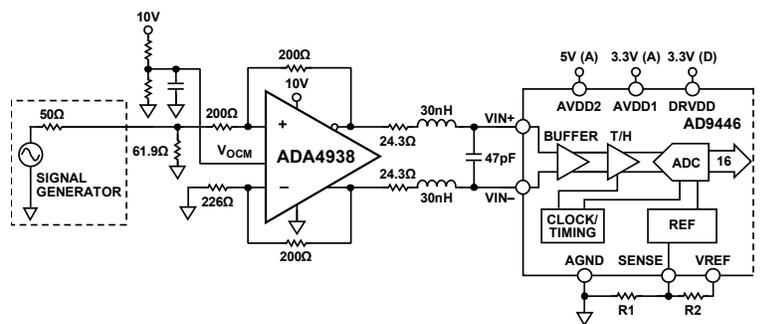
Figure 69. ADA4938-1/ADA4938-2 Driving an AD9446, 16-Bit, 80 MSPS ADC
