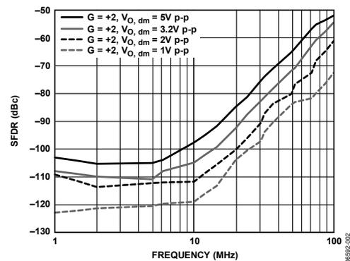
Figure 3. SFDR vs. Frequency and Output Voltage
