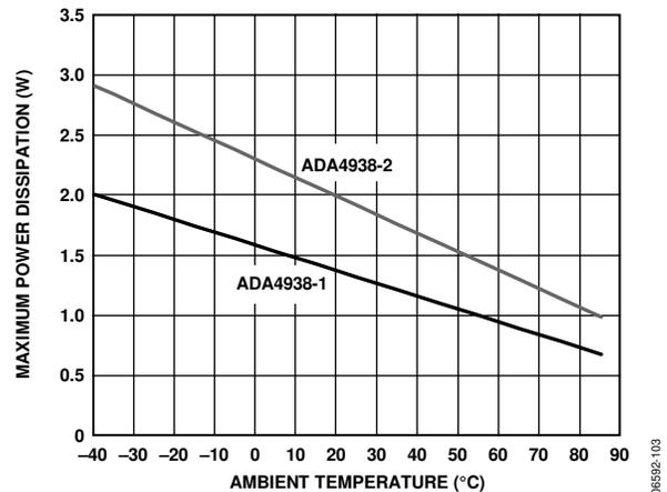
Figure 4. Maximum Power Dissipation vs. Temperature, 4-Layer Board
