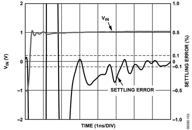
Figure 53. 0.1% Settling Time
