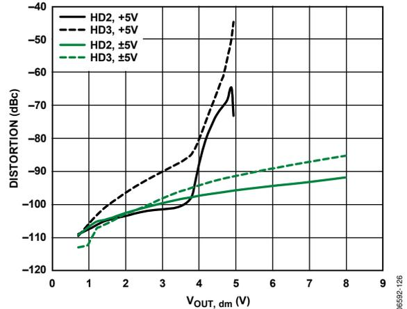
Figure 28. Harmonic Distortion vs.  $V_{OUT}$  and Supply Voltage
