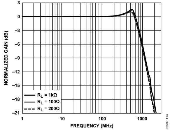
Figure 16. Large Signal Frequency Response for Various Loads
