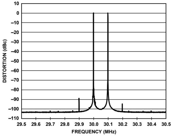
Figure 31. Intermodulation Distortion
