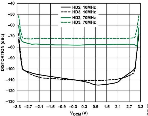
Figure 27. Harmonic Distortion vs.  $V_{OCM}$  and Frequency
