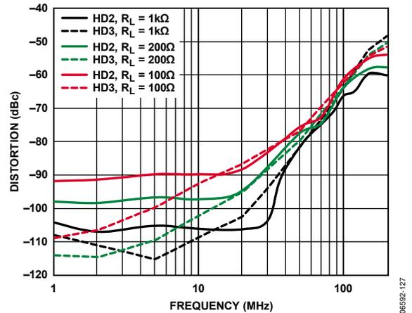
Figure 29. Harmonic Distortion vs. Frequency for Various Loads
