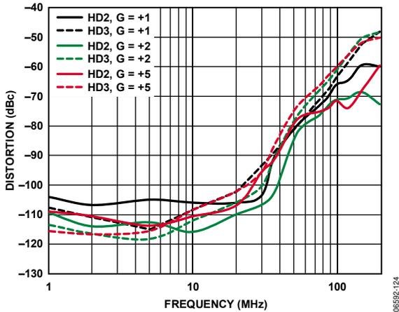
Figure 26. Harmonic Distortion vs. Frequency and Gain
