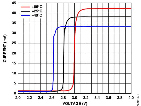
Figure 42. Supply Current vs. Power-Down Voltage and Temperature
