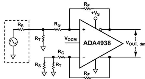
Figure 60. ADA4938-1/ADA4938-2 Configured for Unbalanced (Single-Ended) Input
