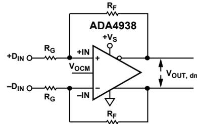
Figure 59. ADA4938-1/ADA4938-2 Configured for Balanced (Differential) Inputs
