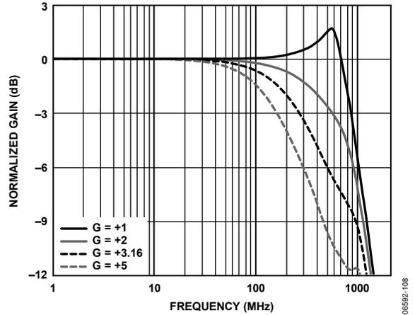
Figure 10. Large Signal Frequency Response for Various Gains
