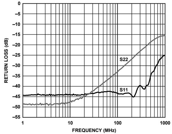
Figure 35. Return Loss ( $S_{11}$ ,  $S_{22}$ ) vs. Frequency
