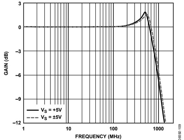
Figure 11. Large Signal Response for Various Supplies
