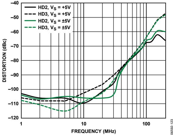
Figure 25. Harmonic Distortion vs. Frequency and Supply Voltage
