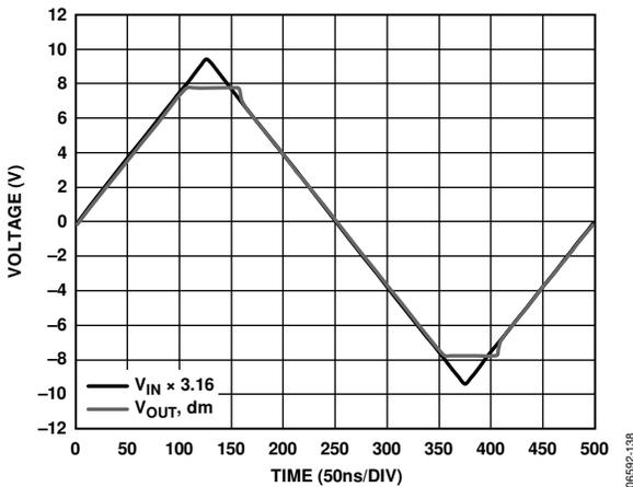
Figure 39. Overdrive Amplitude Characteristics (Triangle Wave Input)
