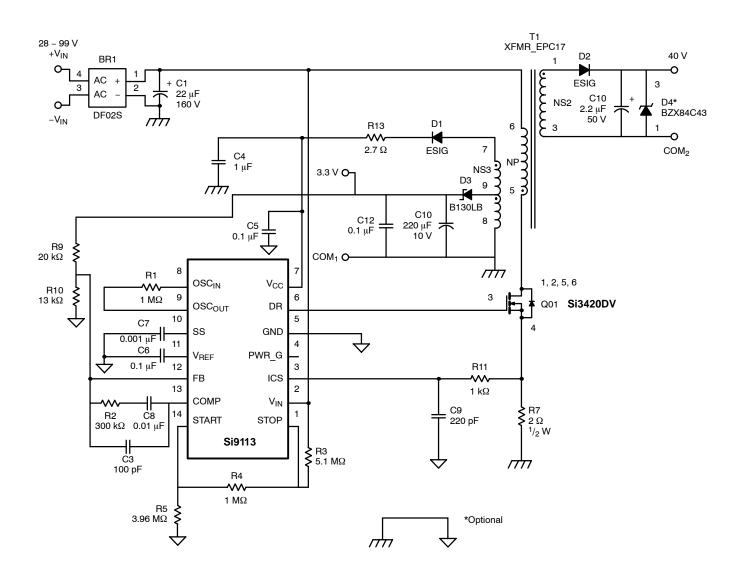
FIGURE 2. Dual Output Flyback Converter with 2% Regulation for 3.3 V (As used on Demo Board—DB1)
