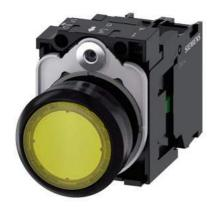
Illuminated pushbutton, 22 mm, round, plastic, yellow, pushbutton, flat, momentary contact type, with holder, 1 NO, LED module with integrated LED 110 V AC, screw terminal
