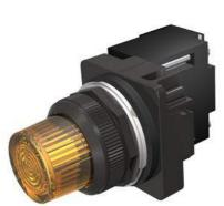
30mm BlackMax, Epoxy Coated Corrosion Resistant Complete Metal Unit Illuminated Indicator Light Full Voltage type, 120V AC/DC LED Lamp, BA9s Glass Lens, Amber UL Listed, CSA Certified NEMA 1,3,3R,4,4X,12,13 & Automotive Standards
