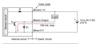
Symbols ... D : Reverse supply polarity protection diode ZD: Surge absorption zener diode Tr : NPN output transistor
