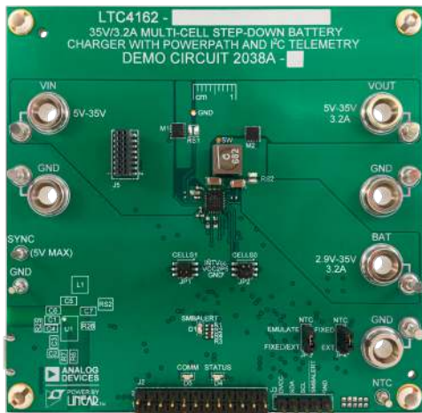
Figure 1. DC2038A is a Battery Charger Demo Board for the LTC4162 Designed to Interface with DC2654A.
