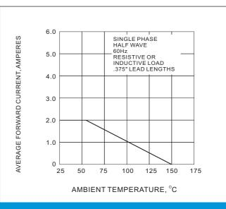
Fig.2 FORWARD CURRENT DERATING CURVE
