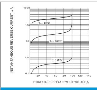
Fig.3 TYPICAL REVERSE CHARACTERISTIC
