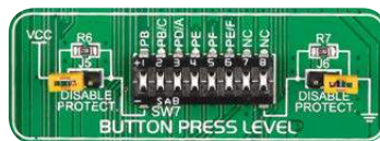
Figure 10-6: Button press level DIP switch (tri-state)
