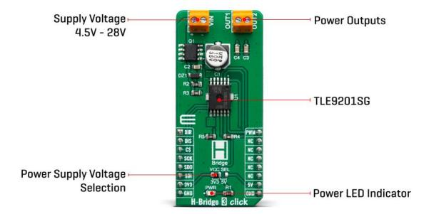
All internal supply voltages are derived from the external VIN conector. A charge pump provides the gate voltage for the high side switches. The output buffer of the digital output SO is supplied by the pin VSO. Therefore the output logic level at SO can be easily configured for 3.3 V or 5 V logic by moving VCC SEL jumper to the respective voltage.
