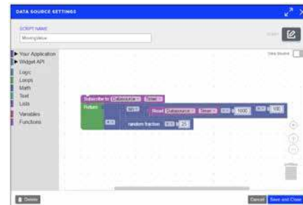
The PowerPro GUI incorporates a powerful script creator function that allows users to write their own process control routines.
