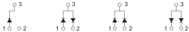
CDBT-40-G Marking Code: 43 CDBT-40S-G Marking Code: 44 CDBT-40C-G Marking Code: 45 CDBT-40A-G Marking Code: 46
