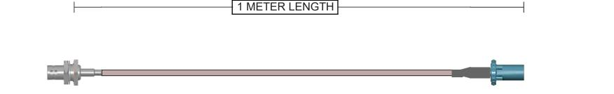
Connector A 112234 BNC Jack Straight Bulkhead - Rear Mount Brass Nickel 50 Ohm RG-316 Continuity/Hi-Pot Connector B 2FA1-NZSP-C01Y1 FAKRA Plug Straight Zinc Nickel + Heatshrink
