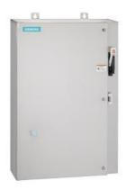
Non-reversing motor starter Size 2 1/2 Three phase full voltage Solid-state overload relay OLRelay amp range 25-100A 110VAC 50HZ / 120VAC 60HZ coil Combination type 100A non-fusible disconnect Encl NEMA type 4X 316 S-steel Water/dust tight non-corrosive Extra-wide enclosure
