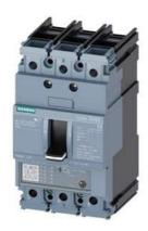
circuit breaker 3VA5 UL frame 125 3-pole, starter protection TM120M, AM, In=100A without overload protection short-circuit protection Ii=3...7 x In cable connection on both sides
