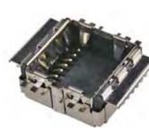
SMIA75, 7.50 by 7.50mm, 16 circuits Through-board, 4.20mm height (Series 105168)
