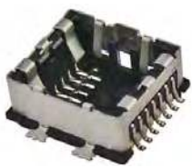
SMIA55, 5.50 by 5.50mm, 14 circuits Through-board, 3.78mm height (Series 105200)
