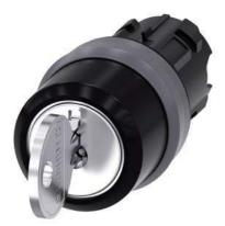
RONIS key-operated switch, 22 mm, round, plastic with metal front ring, lock number SB30, with 2 keys, 3 switch positions I-O-II, latching, actuating angle 2x45°, 10:30h/12h/13:30h, Key removal II, possible special locks: SB31, 421, 455, with laser labeling, upper case and lower case, always upper case at beginning of line
