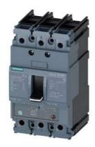
circuit breaker 3VA5 UL frame 125 breaking capacity class S 25kA @ 480 V 3-pole, line protection TM240, ATAM, In=15A overload protection Ir=12A ...15A short-circuit protection Ii=10...20 x In nut keeper kit on both sides
