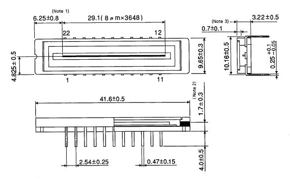
Note 1: Distance between the edge of the package and the first pixel (S1)
