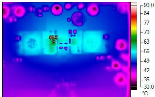
Figure 9. DC3138A Thermal Performance (24V IN , I OUT1 = 15A, I OUT2 = 10A, T A = 25°C, Free Air)
