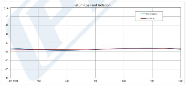
Click the following link (or enter part number in "SEARCH" on website) to obtain additional part information including price, inventory and certifications: 90 Degree Drop-In Hybrid Coupler From 400 MHz to 1,000 MHz Rated to 200 Watts PE2CP1037
