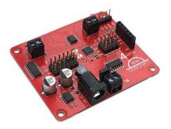
RoboHAT is a complete robotics controller for your Raspberry Pi based mobile robot.
