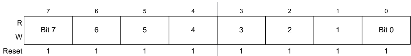
Figure 12-30. PWM Channel Duty Registers (PWMDTY3)
