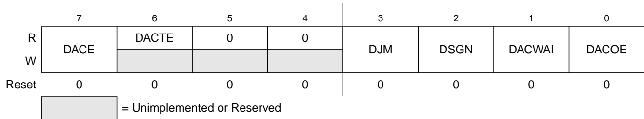
Figure 7-3. DAC Control Register 0 (DACC0)
