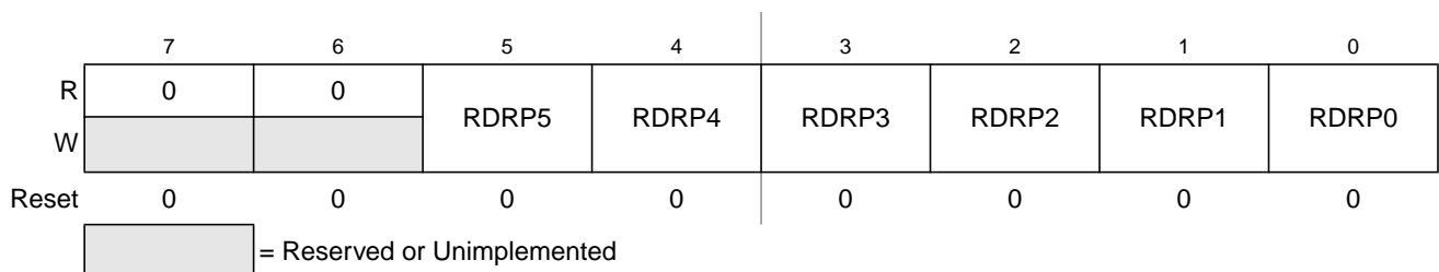
Figure 3-20. Port P Reduced Drive Register (RDRP)
