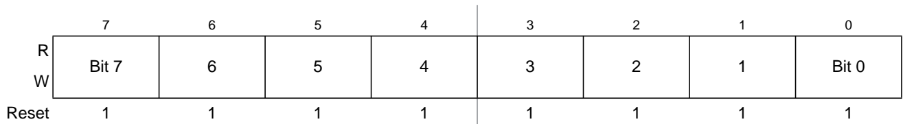
Figure 12-29. PWM Channel Duty Registers (PWMDTY2)
