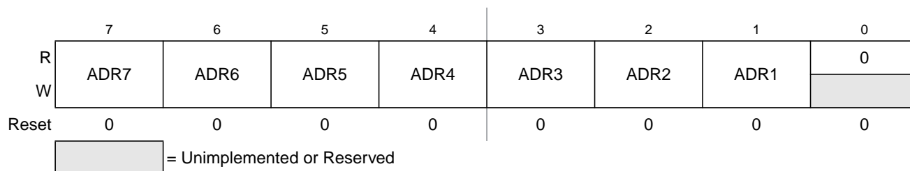
Figure 10-2. IIC Bus Address Register (IBAD)
