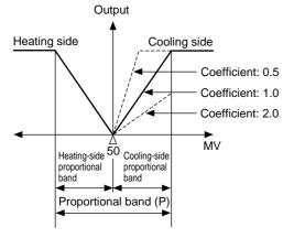
• Before setting the cooling-side proportional band, set the heating-side proportional band to an optimum value. To select the two-position control for the cooling side, set **Laal** to 0.0.
