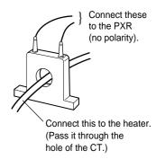
• Connection example for the alarm for heater break (PXR5/9 model)
