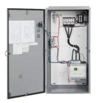
Enclosed soft starter, Controller 3RW44251BC34, Std. duty rating 15HP @230V, Std. duty current rating 51A Control voltage 115Vac Enclosure type NEMA 3/3R Weather proof outdoor use
