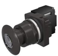
30mm BlackMax, Epoxy Coated Corrosion Resistant Complete Metal Unit Illuminated Push-Pull Operator Full Voltage, 24V AC/DC Incandescent Lamp Mushroom Head Cap Small 1 3/4" (44.5 mm) Metal, Black with Clear Lens 3 Position Momentary UL Listed, CSA Certified NEMA 1,3,3R,4,4X,12,13 & Automotive Standards
