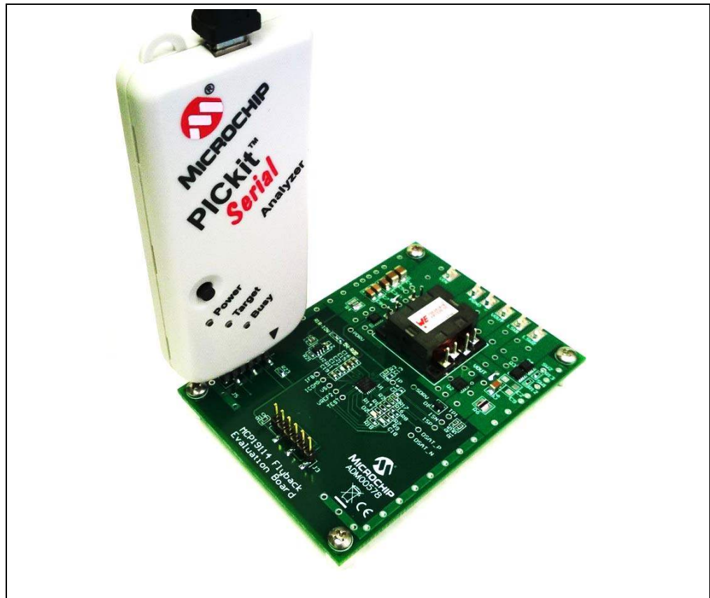
FIGURE 3-1: PICKit Serial Analyzer Connection to the Board.
