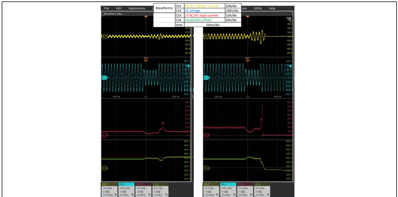
Figure 35 115 V voltage sag from 230 V applied during 100 ms at 380 W (left) and 880 W (right)
