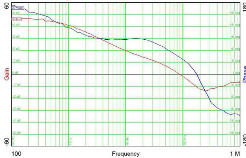
Figure 5. TPS57114EVM Loop-Response Measurement
