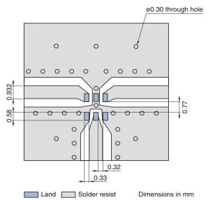
Line width should be designed to match  $50\Omega$  characteristic impedance, depending on PCB material and thickness.
