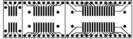
This product is an SOIC to DIP adapter with a twist. These have our patented "ez" technology which means that soldering the surface mount component is simple, and as with all of our "ez" boards, we are the only company with a patented solution for easily soldering surface mount parts. Included in the package are 1.27mm pitch adapter boards for 8 leads, 18 leads, and 28 leads. A standard row of 40 headers has been included as a bonus for your convenience.
