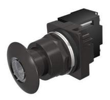
30mm BlackMax, Epoxy Coated Corrosion Resistant Complete Metal Unit Illuminated Push-Pull Operator Full Voltage, 6V AC/DC Incandescent Lamp Mushroom Head Cap Small 1 3/4" (44.5 mm) Metal, Black with Clear Lens 3 Position Pull-Momentary/Push-Maintained UL Listed, CSA Certified NEMA 1,3,3R,4,4X,12,13 & Automotive Standards
