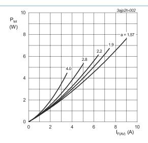
a = form factor =  $I_{F(RMS)}$  /  $I_{F(AV)}$ V<sub>o</sub> = 0.579 V; R<sub>s</sub> = 0.0121  $\Omega$
