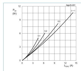
$$\begin{split} & I_{\text{F(AV)}} = I_{\text{F(RMS)}} \times \sqrt{\delta} \\ & V_{\text{o}} = 0.579 \text{ V; R}_{\text{s}} = 0.0121 \text{ }\Omega \\ & \text{Fig. 1. Forward power dissipation as a function of average forward current; square waveform; maximum values; per diode} \end{split}$$
