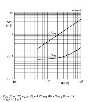
Fig.17 Output admittance as a function of frequency; typical values; amplifier a.
