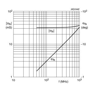
$V_{DS}\left(a\right)=5$  V;  $V_{G2\cdot S}\left(a\right)=4$  V;  $V_{DS}\left(b\right)=V_{G1\cdot S}\left(b\right)=0$  V;  $I_{D}\left(a\right)=12$  mA.
