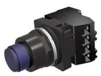
30mm BlackMax, Epoxy Coated Corrosion Resistant Complete Metal Unit PTT / Illuminated Pushbutton Full Voltage, 6V AC LED Lamp Extended Button Plastic Lens, Blue 2 Position Momentary with 1 N.O. - 1 N.C. Heavy Duty Contacts, A600/P600 UL Listed, CSA Certified NEMA 1,3,3R,4,4X,12,13 & Automotive Standards
