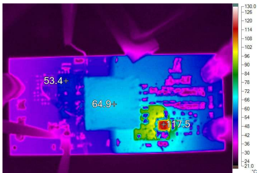
Figure 23. Thermal Image of the Supply in Figure 21 Using a PDS760 Instead of the LT8309 and Synchronous Switch at 5V/5A Output
