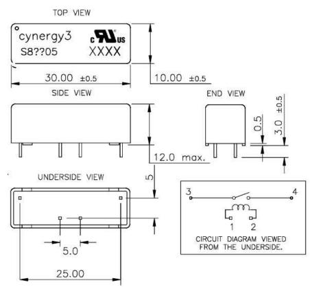
Pins 0.635mm Square ±0.05mm. Pins 1 & 2 Tin over Nickel plated, on CuSn6 Phospher Bronze. Pins 3 & 4 Tin plated on NiFe Nickel Iron. Case Material Nylon. Encapsulant: Epoxy
