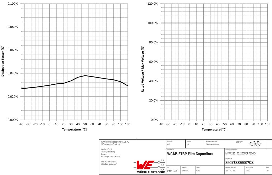
**Rated Voltage vs. Temperature:**
