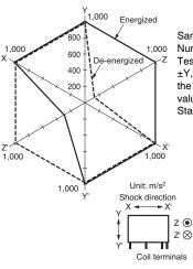
Sample: G6DN-1A Number of Relays: 5 pcs Test conditions: Impose a shock in the ±X,  $\pm$ Y, and  $\pm$ Z directions three times each with the Relay energized to check the shock values that cause the Relay to malfunction. Standard:100 m/s<sup>2</sup>
