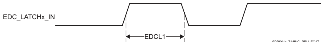
Figure 5-62. PRU-ICSS ECAT LATCHx_IN Timing
