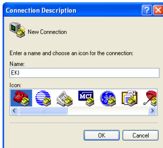
Figure 7.1 Creating a Telnet Connection
