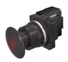
30mm BlackMax, Epoxy Coated Corrosion Resistant Complete Metal Unit Illuminated Push-Pull Operator Full Voltage, 24V AC/DC Incandescent Lamp Mushroom Head Cap Small 1 3/4" (44.5 mm) Metal, Black with Red Lens 3 Position Pull-Momentary/Push-Maintained UL Listed, CSA Certified NEMA 1,3,3R,4,4X,12,13 & Automotive Standards
