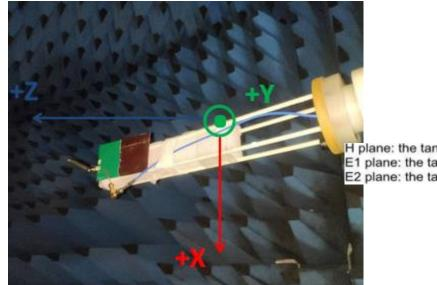
H plane: the tangent of XY E1 plane: the tangent of XZ E2 plane: the tangent of YZ
