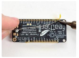
points on each strip, to 'tack' the header in place
