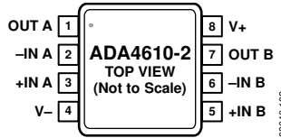
Figure 5. ADA4610-2 Pin Configuration, 8-Lead MSOP (RM Suffix)
